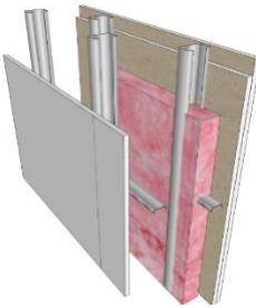
The detail shown here is indicative of a common chase wall constructed with cold-formed steel studs. It depicts two rows of studs where the adjacent studs are connected via a steel track. The presence of the track acts as a gusset which effectively stiffens the studs, thus allowing for thinner width studs to be utilized. This, in turn, increases the chase area.
